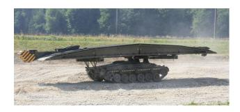
The bridge consists of two track carriers of aluminum alloy. Each track support consists of two end portions and two intermediate portions. It is not a scissors bridge, it is transported in its entire length. The storage beam is mounted between the two tracking beams, which is connected to a hydraulic ram.
