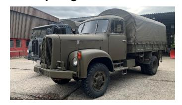
The Saurer 2 DM and Berna 2 VM were among the most popular vehicles, both with drivers and passengers. A heated cabin with three seats was not a normal matter for army vehicles. And the sliding windows in the doors were also very practical. Power-assisted steering, clutch and gear
