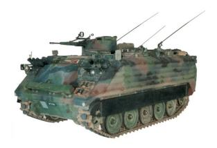
With the introduction of the tank 87 (Leo2), it became necessary to adapt the support vehicles. Among other things, the tank was fitted with Urdan side armour from Israel, additional front armour from FMC (USA), a new engine, a new transmission, a fuel system with two external fuel tanks, neon lights and a rein
