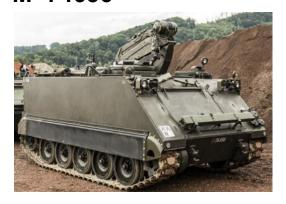
Compared to the normal M113 version, the Crane tank 63 also had a mounted 3-tonne crane and an enlarged roof hatch. It was assigned to the mechanised logistics units and enabled them to carry out repairs in the field.
