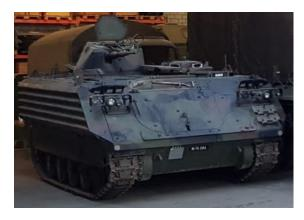
With the introduction of the tank 87 (Leo2), it became necessary to adapt the support vehicles. Among other things, the tank was fitted with Urdan side armour from Israel, additional front armour from FMC (USA), a new engine, a new transmission, a fuel system with two external fuel tanks, neon lights and a rein
